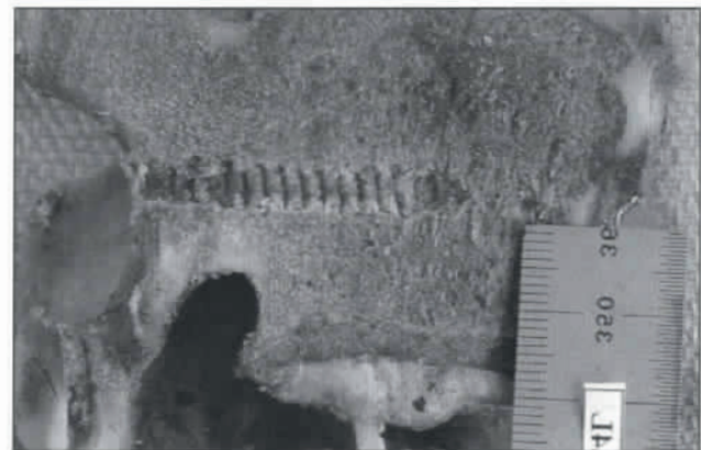
Figure 4A: Sagittal view of a typical specimen after screw failure
