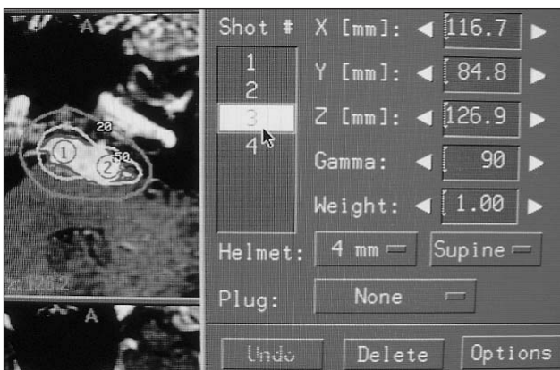
Figure 6: A picture from the monitor at the beginning of the treatment plan. The red line indicates the target and the yellow line shows 50% isodose (50% of the maximum dose) line produced by 3 shots. The yellow line indicates the active radiation field for the target. The green line shows the border that receives 20% of the maximum dose and it is generally used to observe the dose that the important structures receive. The coordinates of the third shot can be followed on the right box.
