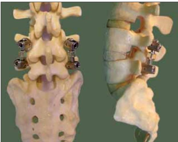
**Figure 4:** Agile rod system with safinaz dynamic screws in a saw bone.
