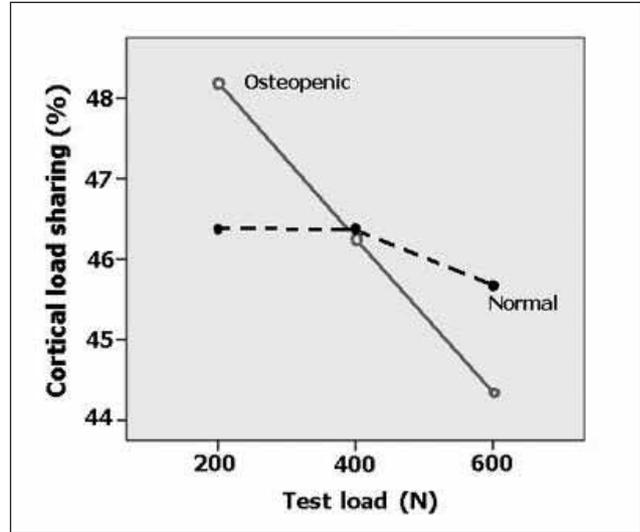
**Figure 5:** The relationship between load sharing and test load. The osteopenic vertebrae showed significantly lower cortical load sharing ratios as the load increased. The test was performed at 1 mm/sec test speed.
