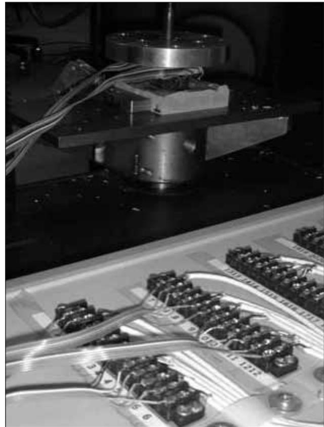
Figure 2: A view of the experiment design. The wires protruded from the specimen's strain gages were connected to the signal conditioning equipment.
