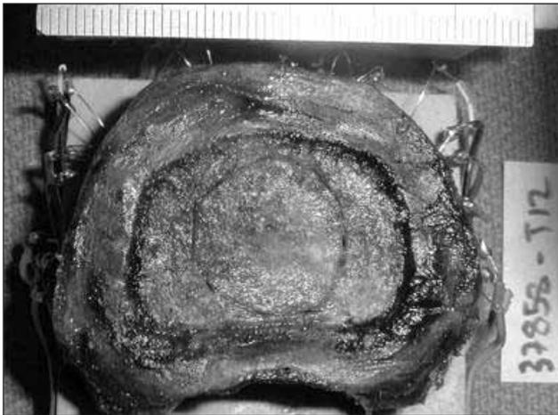
**Figure 3:** The bottom view of the vertebra after creation of a window at the center of endplate to reach trabecular bone. Note that an area of the central 25% of the trabecular bone was determined and carved.
