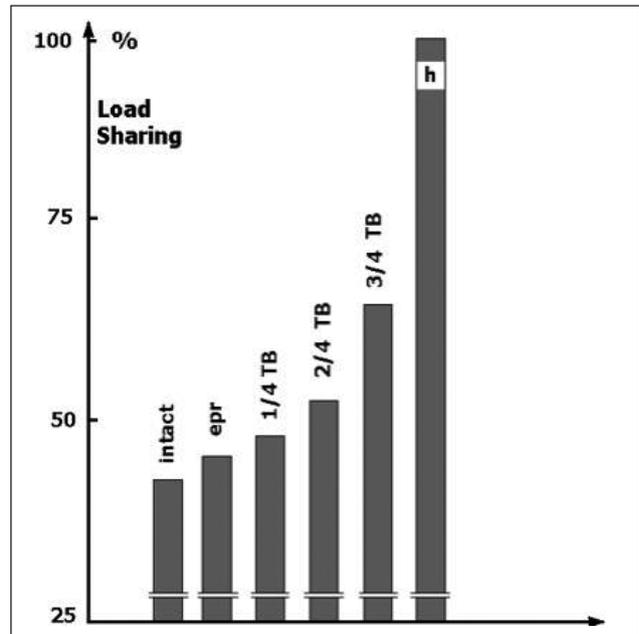
**Figure 4:** Cortical strains after stepwise removal of trabecular centrum. While the amount of increase of load sharing was relatively small after removal of first two quarters (middle of the vertebrae: 1/4 TB and 2/4 TB), it was substantial after outer two quarters of the trabecular bone vanished (3/4 TB and h step). (epr: end-plate removal, TB: trabecular bone, h: hollowed, total trabecular bone removal).
