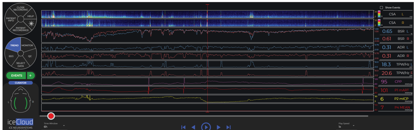
Figure 2: Image from iCEWav demonstrating an example of the quantitative electroencephalography (EEG) values converted from the raw EEG patterns that the system collects. These incorporate similar quantitative variables as used in traditional scalp EEG. BSR: Burst suppression ratio, CSA: Compressed spectral array, ADR: Alpha-delta-ratio, TPW (total power)—and can incorporate traditional hemodynamic variables— CPP: Cerebral perfusion pressure, mART: Mean arterial pressure, ICP: Intracranial pressure, P4: Brain oxygen.
