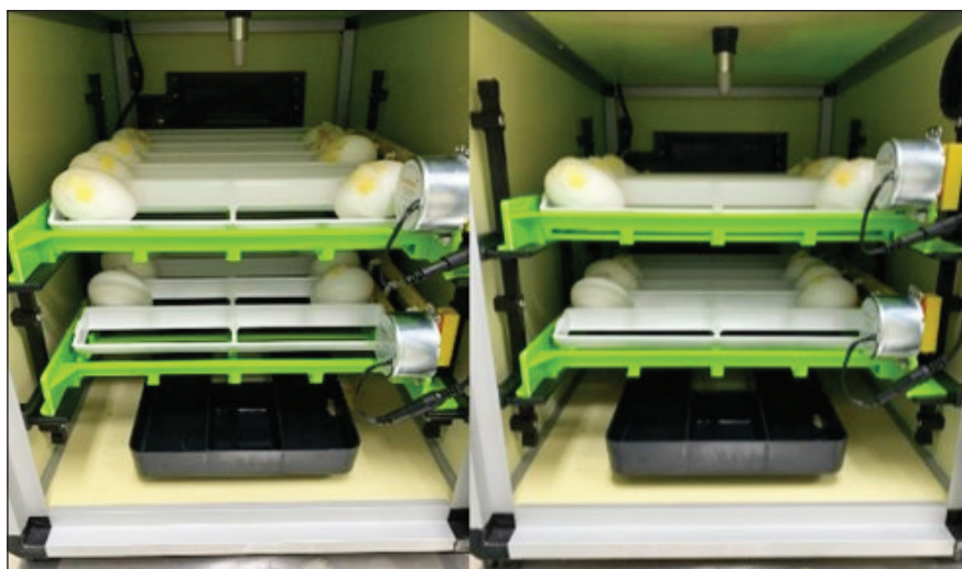
Figure 1: The arrangement of special pathogen-free (SPF) eggs within the incubator. The pointed edges of SPF eggs project downwards.
