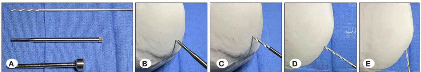
**Figure 1:** **A)** Commonly used drill (top), Cosman-Roberts-Wells (CRW) drill guide tube (middle), and Ad-tech drill sleeve guide (bottom) for insertion of Stereotactic electroencephalography (SEEG) electrodes. **B)** Drill minimally protruding beyond guide tube resulting in little drill flex. **C)** Drill protruding beyond the guide tube resulting in more drill flex. **D)** Ideal orthogonal approach angle. **E)** Oblique drill approach angle.
