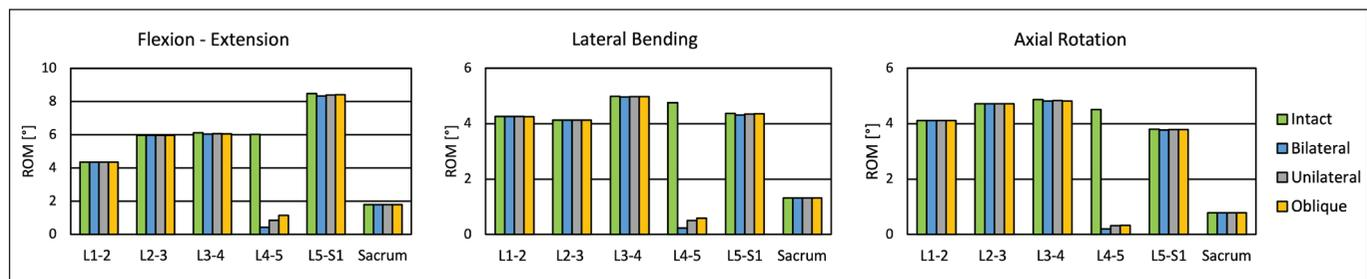
**Figure 2:** Comparison of the global range of motion (degree) of uninstrumented spine and three rod configurations (bilateral, oblique and unilateral) under flexion-extension, lateral bending and axial rotation.
