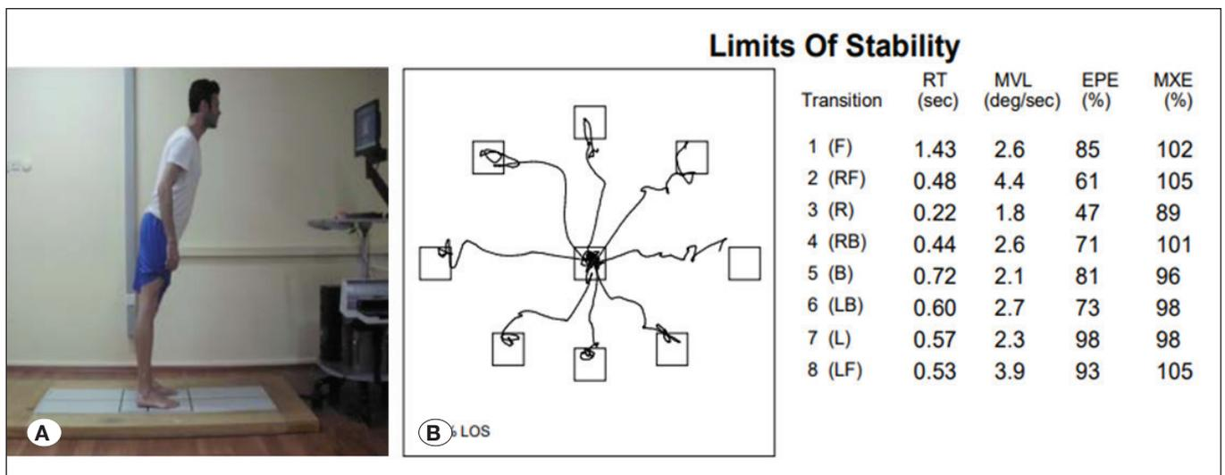
**Figure 3:** For dynamic balance evaluation, the volunteer was asked to shift his center of pressure (COP) by reaching in the direction of different targets as soon as possible after the visual signal was triggered on the computer screen (A). Test result of dynamic balance assessment (Limits of stability test) (B).
