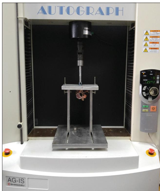
**Figure 3:** Pullout test setup using L4 ovine vertebrae (AG-I 10 kN, Shimadzu, Japan).
