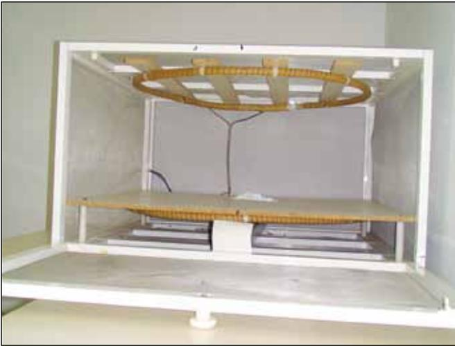
**Figure 3:** Four different brands of programmable CSF shunts were exposed to the magnetic field generated by our apparatus described above coil for 5 minutes.
