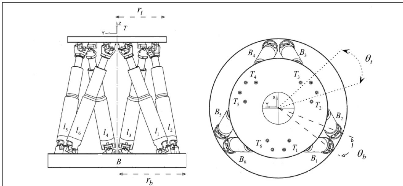
**Figure 1:** Kinematic configuration of the SP.
