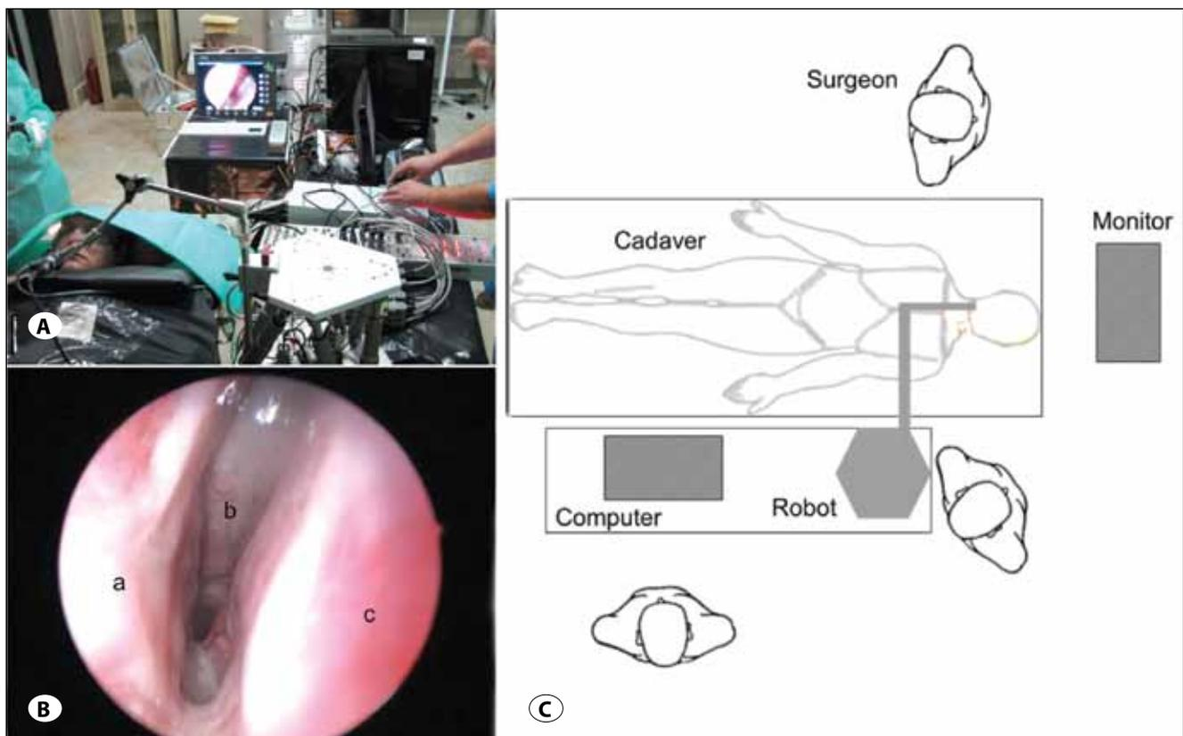
**Figure 4:** A, C) The pictures show the orientation and position of the robotic endoscope holder system in the operating room. B) Anterior wall of sphenoid sinus was visualized during cadaveric dissection (a. nasal septum, b. anterior wall of the sphenoid sinus, c. middle concha).
