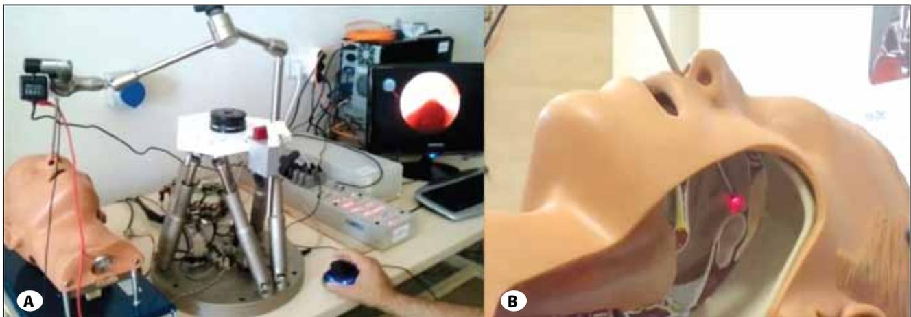
**Figure 3: A)** The picture shows the attachment of the endoscope to the Stewart Platform. **B)** Insertion of the endoscope into the right nostril of the artificial model.
