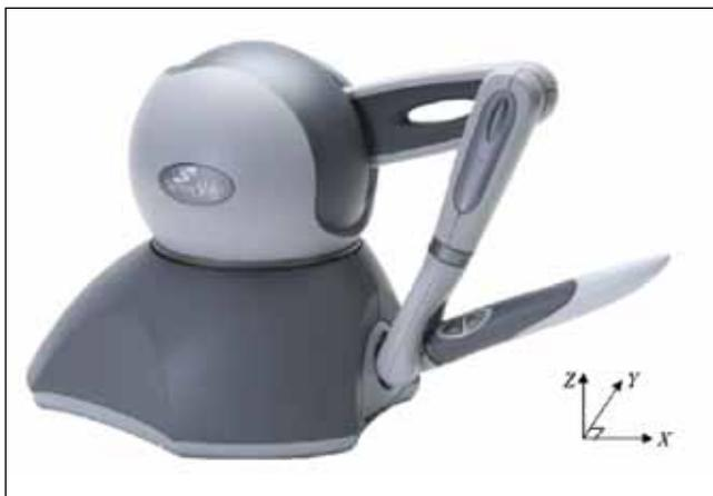
**Figure 2:** Phantom Omni Haptic.
