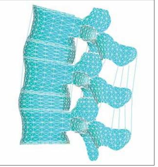
Figure 1: Normal finite element model of L3-5.
