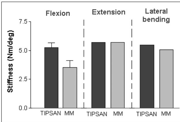
**Figure 9:** Comparison of TIPSAN and Moss-Miami stiffnesses at flexion, extension, and lateral bending modes. The TIPSAN system was stiffer than Moss-Miami ( $p=0.039$ ) at flexion mode. There were no statistically significant difference at extension and lateral bending modes.
