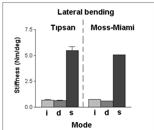
**Figure 8:** Stiffnesses at intact, destabilized and instrumented modes at lateral bending for TIPSAN and Moss-Miami instrumentations. While the destabilization process did not affect specimen stiffness, stabilization significantly increased the stiffness (p<0.0001) for both of the devices (i=intact, d=destabilized, s=stabilized).
