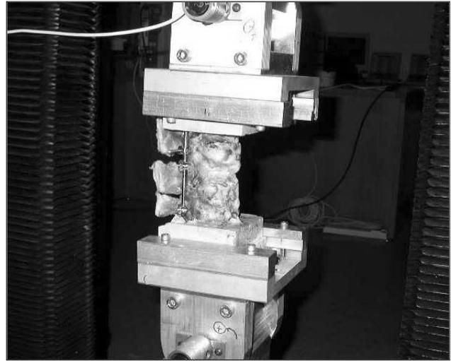
Figure 5: Testing Procedure in MTS machine
