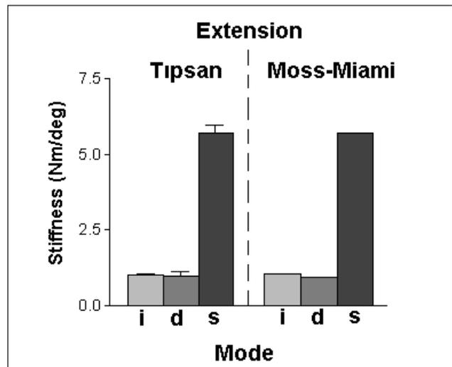
**Figure 7:** Stiffnesses at intact, destabilized and instrumented modes at extension for both devices. While the destabilization process did not affect specimen stiffness, stabilization significantly increased the stiffness (p<0.0001) for both of the instruments (i=intact, d=destabilized, s=stabilized).
