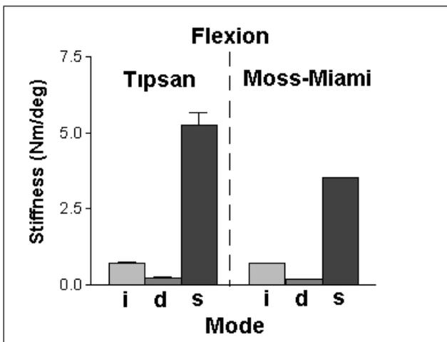
**Figure 6:** Stiffnesses at intact, destabilized and instrumented modes at flexion for TIPSAN and Moss-Miami instrumentations. The destabilization process significantly lowered specimen stiffness, and stabilization (i.e., instrumentation) significantly increased the stiffness (p<0.0001) for both of the instruments (i=intact, d=destabilized, s=stabilized)
