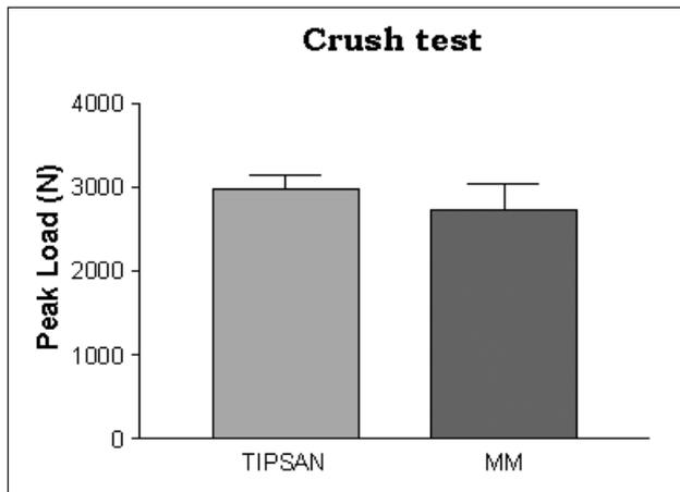
**Figure 10:** Comparison of TIPSAN and Moss-Miami peak loads in the strength (=crush) test. The results are similar.
