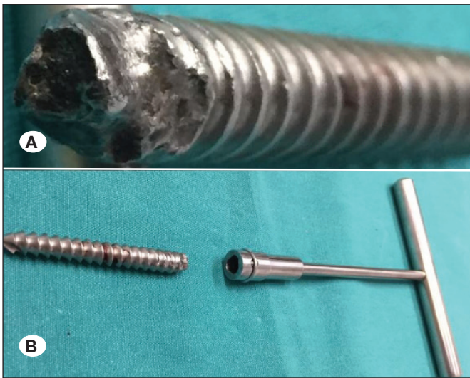
Figure 1: A) Shaping the broken screw head with the help of a high-speed drill. B) Compatibility of the removed broken screw with the extractor
