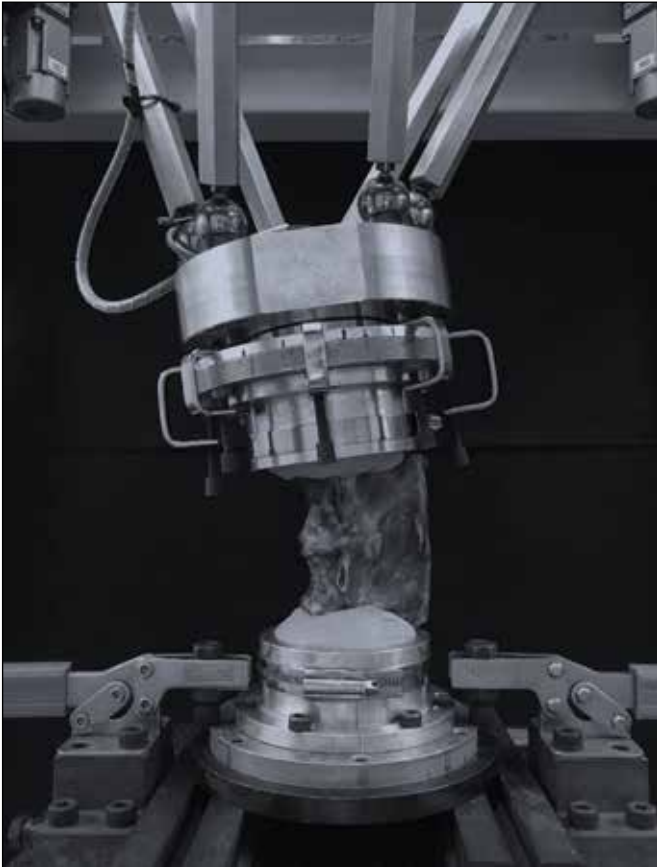
Figure 2: A 6-axis material testing machine during flexion test with the intact model.
