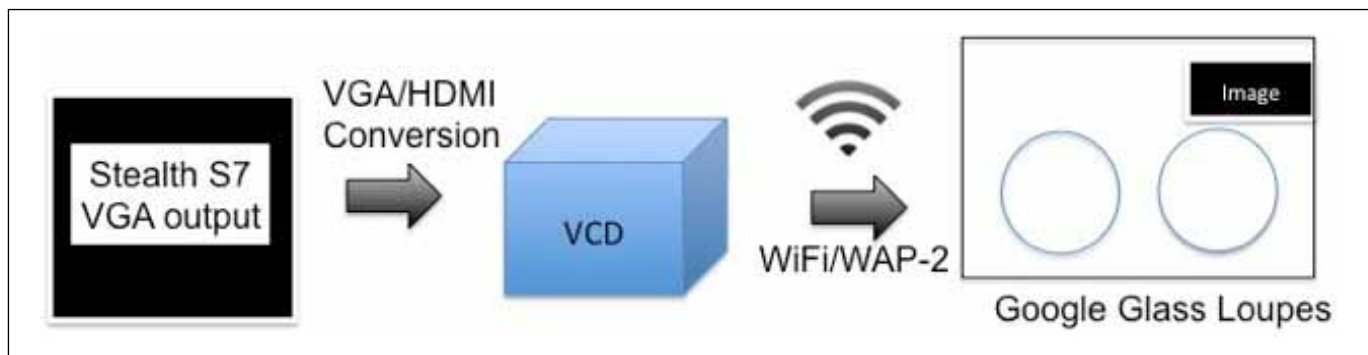
Figure 1: Schematic diagram of the video-capture and streaming system for head-up Google glass display of Stealth S7 image-guidance. VGA–video graphics array, HDMI–high-definition multimedia display, VCD–video capture device, WAP2–Wi-Fi protected access 2. Location of Google Glass image output in relation to loupe magnifying field (circles) demonstrated.
