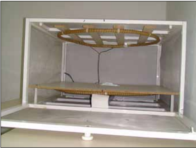
Figure 3: Four different brands of programmable CSF shunts were exposed to the magnetic field generated by our apparatus described above coil for 5 minutes.
