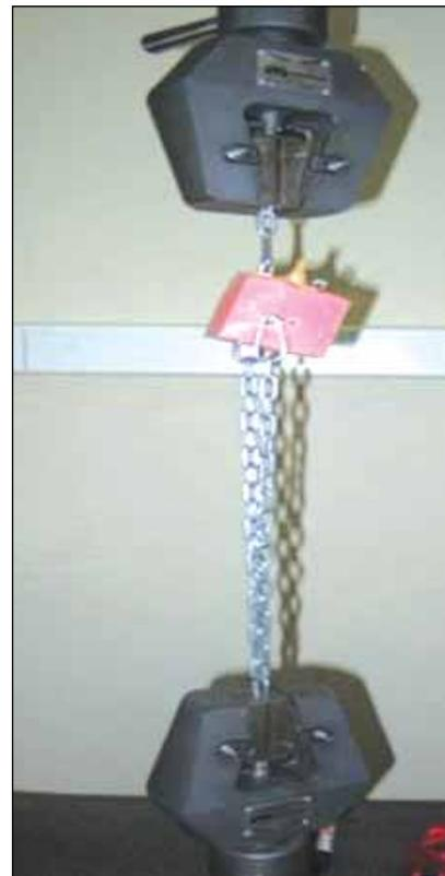
**Figure 3:** Pullout test of the specimen with the Instron 850 biomechanical testing machine.
