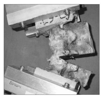
Figure 3: Testing of a destabilized specimen at the flexion mode
