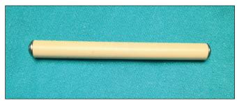
Figure 2: Polyetheretherketone (PEEK) rod.
