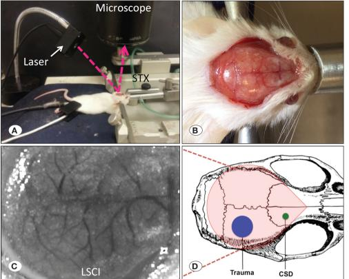
Figure 2: Setup for laser speckle contrast imaging. A) Laser is reflected on the exposed skull and captured via microscope and camera. B) Head is fixed in the stereotaxic frame (STX). C) Laser speckle contrast imaging allows visualization of cortical vasculature and relative regional CBF changes. D) Trauma impact is applied on the right parietal cortex while a small frontal burr hole was used to induce CSD with a pinprick.
