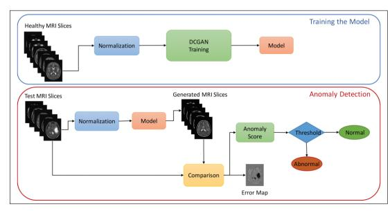
**Figure 2:** Diagram summarizing structure of proposed anomaly detection framework.
