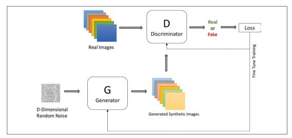
**Figure 1:** Diagram summarizing structure of generative adversarial networks.
