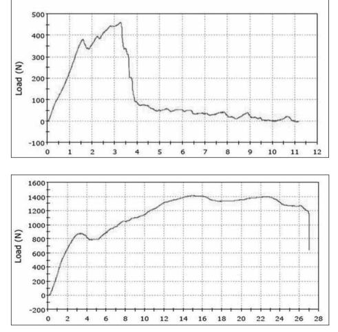
**Figure 4**: Graph showing pullout values of the screw without *"Dubel"*. The peak pullout value was 456.09102 Newton for this specimen. \*The X axis is time (t)
