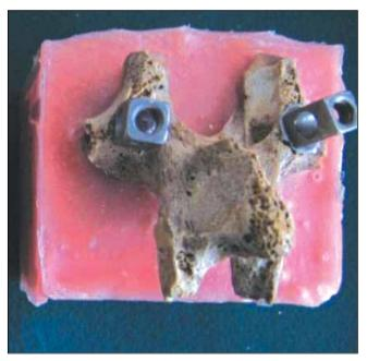
**Figure 2:** Specimen embedded in acrylic cast. Right pedicle has screw with "*Dubel*" and left pedicle has screw only.
