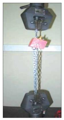
Figure 3: Pullout test of the specimen with the Instron 850 biomechanical testing machine.
